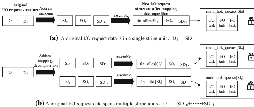
Fig. 10 An original I/O request address mapping and decomposition process
